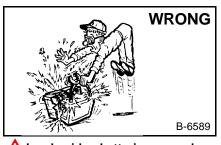
Lead-acid batteries produce flammable and explosive gases.
