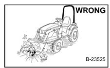
Disconnecting or loosening any hydraulic tubeline, hose, fitting, component or a part failure can cause loader arms to drop.
