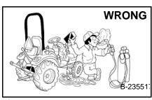
A Stop, cool and clean engine of flammable materials before checking fluids.
