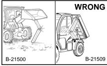
Never work on the machine with lift arm or cargo box up unless supported by an approved support device. Replace if damaged.
