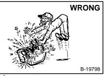
Lead-acid batteries produce flammable and explosive gases.
