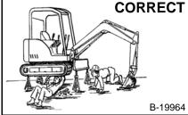
Use the correct procedure to lift and support the excavator.
