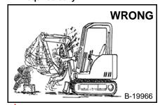
Always lower the bucket and blade to the ground before doing any maintenance.
