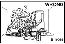
Have good ventilation when welding or grinding painted parts. Wear dust mask when grinding painted parts. Toxic dust and gas can be produced.
