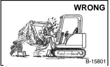
Always lower the bucket and blade to the ground before doing any maintenance.
