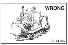
Stop, cool and clean engine of flammable materials before checking fluid.
