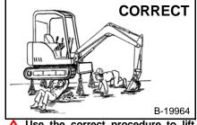
Left Use the correct procedure to lift and support the excavator.
