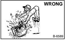
Lead-acid batteries produce flammable and explosive gases. Keep arcs, sparks, flames and tobacco away lighted from
