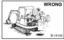
Keep body, jewelry and clothing moving away from parts, electrical contact, hot parts and exhaust.
