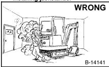
Vent exhaust to outside when engine must be run for service. Exhaust system must be tightly sealed. Exhaust Fumes can kill without warning.
