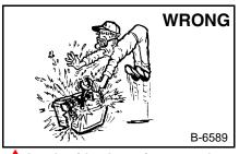
Lead-acid batteries produce flammable and explosive gases.
