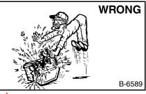
Lead-acid batteries produce flammable and explosive gases.
