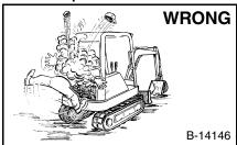
Stop, cool and clean engine of materials flammable before checking fluids.
