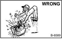
Lead-acid batteries produce flammable and explosive gases. Keep arcs, sparks, flames and lighted tobacco away from
