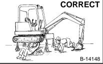
Use the correct procedure to lift and support the excavator. Always lift the blade fully before installing jackstands.
