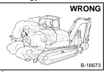
Always lower the bucket and blade to the ground before doing any maintenance.
