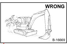
Keep body, jewelry and clothing from moving parts, electrical contact, hot parts and exhaust.
