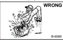
Lead-acid batteries produce flammable and explosive gases.
