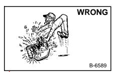
Lead-acid batteries produce flammable and explosive gases.
