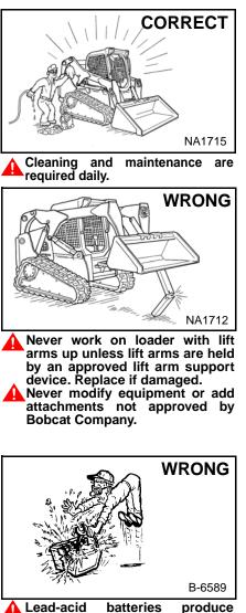
Lead-acid batteries produce flammable and explosive gases. Keep arcs, sparks, flames and lighted tobacco away from batteries. Batteries contain acid which burns eyes or skin on contact. Wear protective clothing. If acid contacts body, flush well with water. For eye contact flush well and get immediate medical attention.
