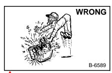
Lead-acid batteries produce flammable and explosive gases.
