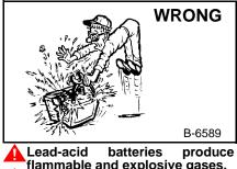
flammable and explosive gases. Keep arcs, sparks, flames and lighted tobacco away from batteries.
