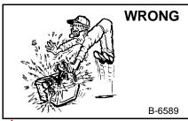
Lead-acid batteries produce flammable and explosive gases.
