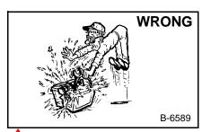
Lead-acid batteries produce flammable and explosive gases.
