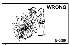
Lead-acid batteries produce flammable and explosive gases.
