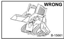
Disconnecting or loosening any hydraulic tubeline, hose, fitting, component or a part failure can cause lift arms to drop. Do not go under lift arms when raised supported bv approved lift arm support device. Replace it if damaged.
