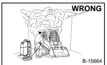
good ventilation Have welding or grinding painted parts. Wear dust mask when grinding painted parts. Toxic dust and gas can be produced.
