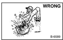
produce Lead-acid batteries flammable and explosive gases. Keep arcs, sparks, flames and lighted tobacco away
