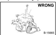
Stop, cool and clean engine of flammable before materials checking fluids.
