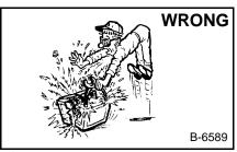
Lead-acid batteries produce flammable and explosive gases.
