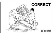
Use the correct procedure to lift to lower operator cab.
