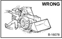
Keep body, jewelry and clothing away from moving parts, electrical contact, hot parts and from moving exhaust
