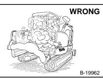
Stop, cool and clean engine of flammable materials before checking fluids.
