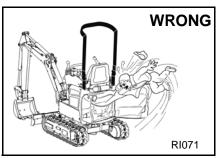
Keep body, jewellery and clothing away from moving parts, electrical contact, hot parts and exhaust.
