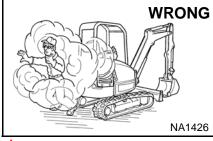
Vent exhaust to outside when engine must be run for service.
