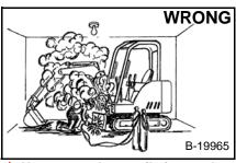
Have good ventilation when welding or grinding painted parts.
