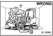
Have good ventilation when welding or grinding painted parts.
