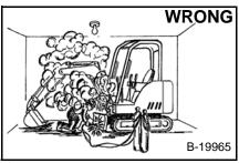
good ventilation welding or grinding painted parts. Wear dust mask when grinding painted parts. Toxic dust and gas can be produced.
