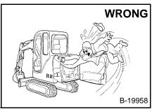
Keep body, jewelry and clothing away from moving parts, electrical contact, hot parts and exhaust.
