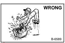
Lead-acid batteries produce flammable and explosive gases.
