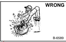
Lead-acid batteries produce flammable and explosive gases.
