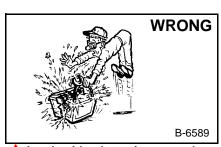
Lead-acid batteries produce flammable and explosive gases.
