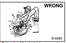
Lead-acid batteries produce flammable and explosive gases.
