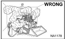
Have good ventilation when welding or grinding painted parts.
