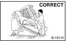
Lise the correct procedure to lift to lower operator cab.
