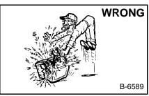
Lead-acid batteries produce flammable and explosive gases.
