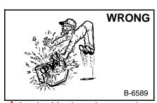
Lead-acid batteries produce flammable and explosive gases.
