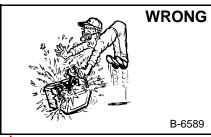
Lead-acid batteries produce flammable and explosive gases.
