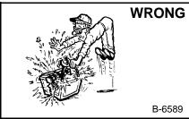
Lead-acid batteries produce flammable and explosive gases.
