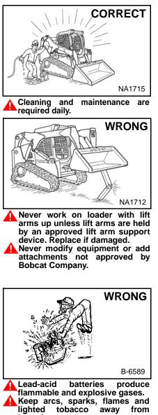
batteries. Batteries contain acid which burns eyes or skin on contact. Wear protective clothing. If acid contacts body, flush well with water. For eye contact flush well and get immediate medical attention.
