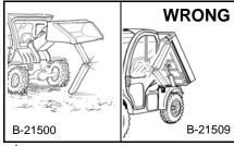
Never work on the machine with lift arm or cargo box up unless supported by an approved support device. Replace if damaged.
