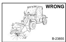
Disconnecting or loosening any hydraulic tubeline, hose, fitting, component or a part failure can cause lift arm or implement to drop. Do not go under lift arm when raised unless supported by an approved lift arm support device or under raised implement unless it is properly supported. Replace if damaged.
