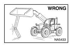
handler with boom up unless boom is held by an approved boom stop. Replace if damaged.
